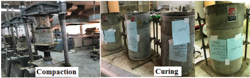
Fig. 4. Compaction and curing of CBR specimens
