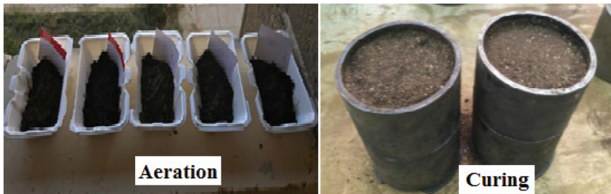
Fig. 3. Aeration of asphalt mixture and curing of specimens
