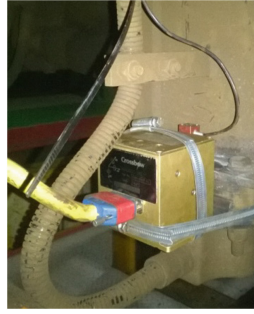
Fig. 1. Bogie mounted gyrometer and accelerometer
