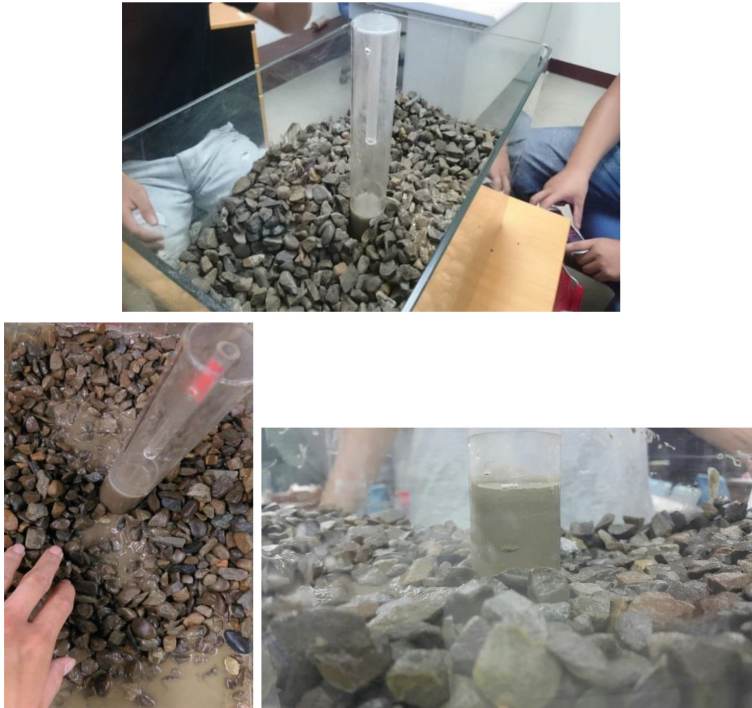
Fig. 10. Different view of the uplift floater by cyclic loading
